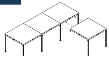
Upon completion of the back row, begin the second row with one section and two legs as shown in Step 4- B, C & D.
